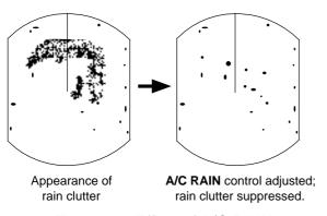
Figure 2-3 Effect of A/C RAIN
